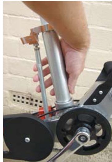
ABOVE: First squeeze the locking bar behind the seatpost – this then drops down.
