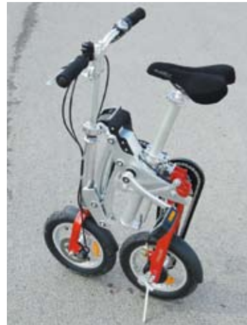
ABOVE: First squeeze the locking bar behind the seatpost – this then drops down.
